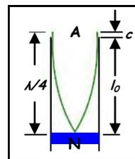
In this first resonance position the air column is vibrating in its **fundamental mode** with a **node (N)** at the closed end and an **antinode (A)** at a distance (**c**) above the open end. 'c' is called the '**END CORRECTION**'. Then :
