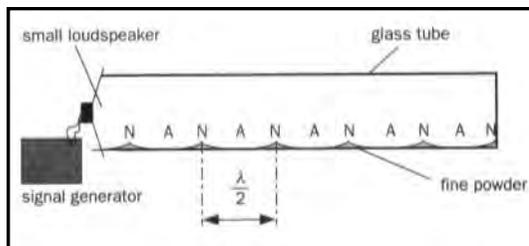
When the frequency of the sound from the loudspeaker is steadily increased from a low value, the sound produced becomes louder at certain frequencies. These loudness peaks are caused when the air column in the tube is set into resonant vibration by the vibrating loudspeaker cone.
