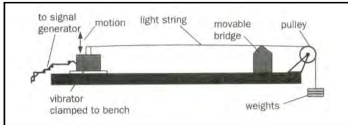
The apparatus shown in the diagram above (Known as **MELDE'S apparatus**) can be used to study the behaviour of vibrating strings.
