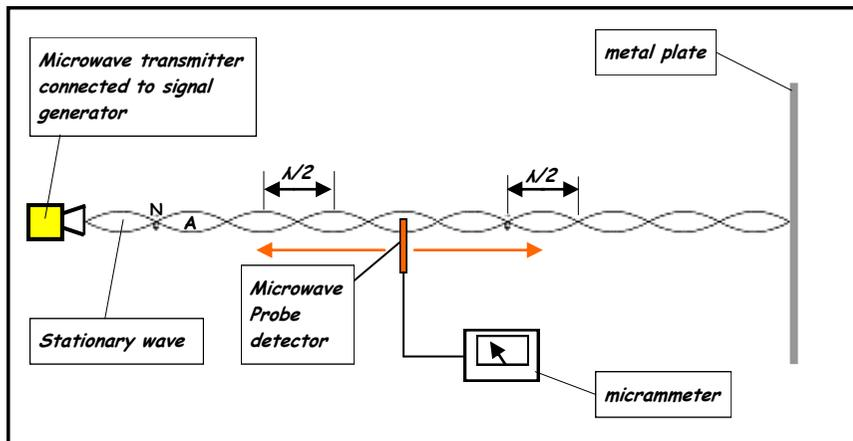
A microwave transmitter connected to a signal generator is used to direct microwaves at a metal plate as shown in the diagram above. The microwaves are reflected from the metal plate and superposition between the incident and reflected waves can produce a **stationary wave**.
